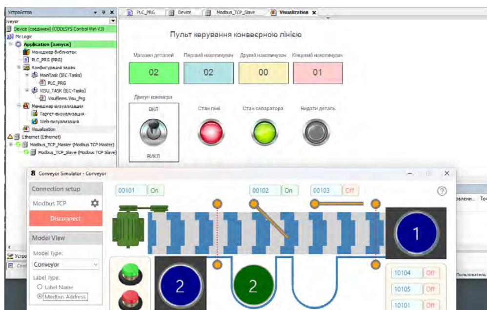
Fig. 9. An example of the program interface and virtual layout in the process of executing a technological program
