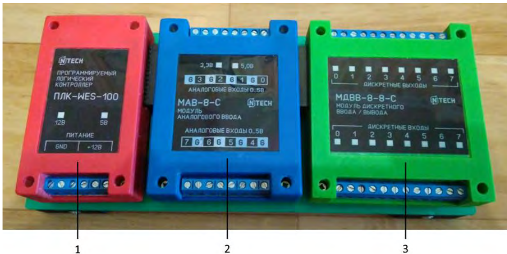
Fig. 1. Exterior of the modular PLC: 1 – central processing unit based on the Raspberry mini-PC; 2 – analog input module; 3 – discrete I/O module
