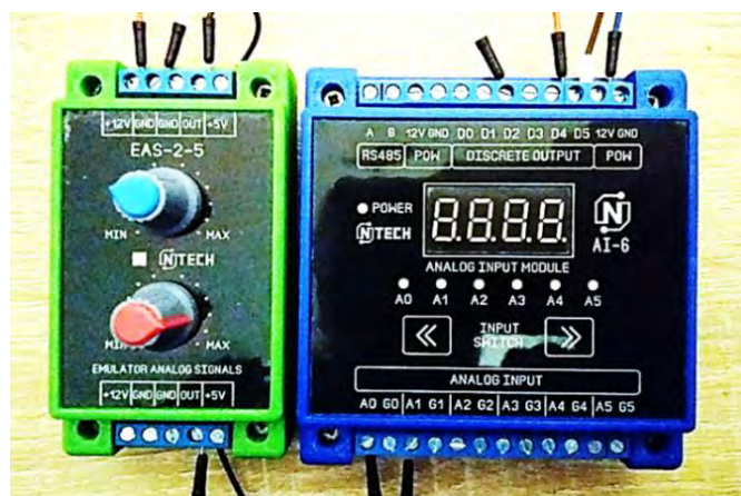
Fig. 2. Expansion module for converting analog signals
