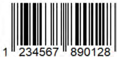
Fig. 2. An example of a message in the form of an EAN-13 barcode
