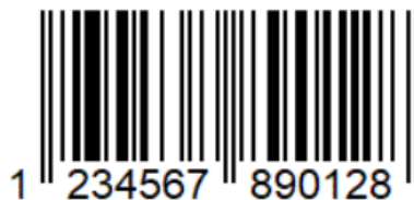
Fig. 2. An example of a message in the form of an EAN-13 barcode
